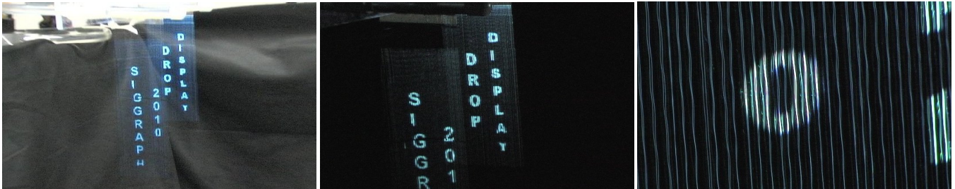
(b) Zooming in on text (15 drops per second): Because the drops oscillate as they fall, they appear as wiggly lines when viewed close up. But because they are generated with the same initial oscillation, each drop distorts in the same way as it falls, and the wiggles appear stationary.
